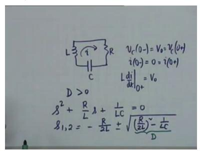
This circuit an RLC series circuit RLC in which V c 0 - = some voltage V0, the current in the circuit if this is the direction of the current i of 0 - = 0, and by continuity of capacitor voltage and inductor current we know that this should be true. The other initial condition is that L di dt at t = 0 + should be equal to V 0, and if this initial conditions we have solved the circuit for the case when the D the discriminant is greater than 0, if you recall the characteristic equation of the
