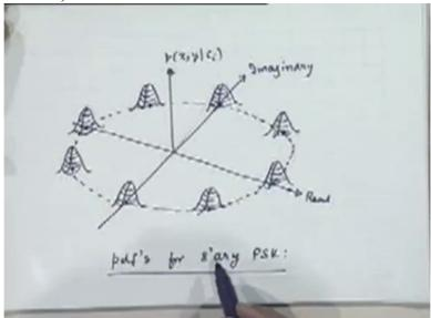
These are the 8 points in the signal constellation diagram lying on a circle, right and around each of these mean values we will have a two dimensional Gaussian s d function coming up which describes the density function of u sub l,
