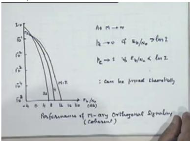
of this error probability, Ok. I plotted here for E B against N zero for different values of N. So as you can see, as you increase the value of M, the curve tends to become lower and lower provided you are above some
