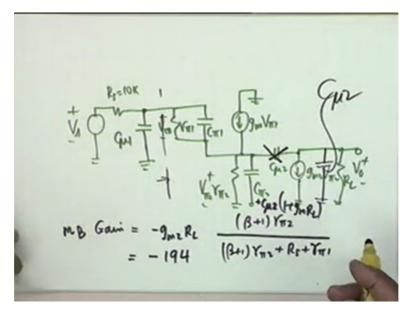
Let us draw the equivalent circuit, it does not take much time. VS, RS which is 10k, then what do you have from here to ground, from here to ground what do you have? If you look at the equivalent circuit, R pi, not to ground, to ground I am asking, to ground is there any element?
