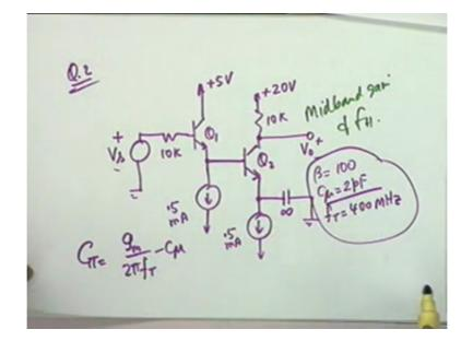
The 2<sup>nd</sup> problem, the 2<sup>nd</sup> problem is that of CE, I am sorry CC CE combination, draw the circuit with me. VS, 10 K, Q1, all transistors are biased by a current generator, this is biased by a current generator and this goes to the next page, that is Q2, this is also biased by a current generator, 0.5 milliamperes. And then you have come in order that this is not floating, you apply a capacitance, a short-circuit, a bypass capacitance.
