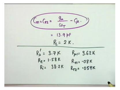
gm is 40 millimho and Omega T is 2 pi times 400 times 10 to the 6, from that you subtract C mu and the result is 13.9 picofarads. You recall this formula, many a times C pi shall not be given, what is given is FT but CU is required. If C mu is not given, what will you do? Ignore it, if it is not given, ultimately be 0. Good strategy, yes. In addition, what else do you need, you need RL, RL is given as 2K.
