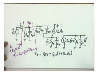
I have a V S, RS, then RB, C mu 1, R pi 1, C pi 1, voltage is V pi 1, this goes to RE and a capacitance CT where CT, what do we do with R pi 2, R pi 2 is combined with RE 1. Okay, CT is C mu, I beg your pardon, C pi 2 plus C mu 2, 1+ gm RL. Okay. This is V pi 2 and then you have the gm v pi 2, then RL, gm 2.
