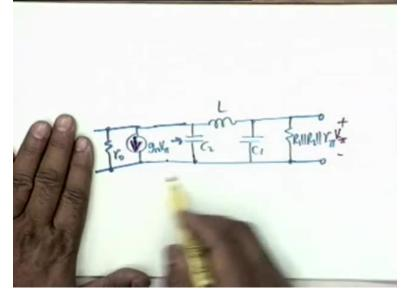
And therefore if you open the loop, you have C2, L, C1, then it should be terminated in R1 parallel R2 parallel R pi. Okay? Now whatcomes here? Here comes the RF choke. For all practical purposes can be taken as of infinite impedance as compared to the impedanceoffered here okay and therefore that we can ignore. We have a current generator, GMV pi in parallel with R not. This is what gives the output impedance. And you see, the output impedance is far from being negligible.
