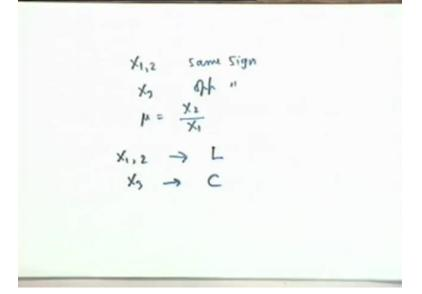
So the condition of oscillation is that X12, same sign, that is both are either inductors or both are capacitances. X3 of opposite sign and mew should be equal to X2 by X1. These are the conditions of oscillation. Accordinglywe can have 2 different types of oscillations. For example, X1 and X2, suppose both are inductances, L, then X3 should be a capacitance. Agreed? Let us look at the circuit.
