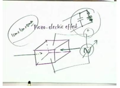
P I E Z O electric effect. And this effect is as simple as this. If you have a block, let us say rectangular block of the Crystal which is properly cut and suppose you apply mechanical pressure to 2 of these faces, okay, suppose you apply mechanical pressure.
