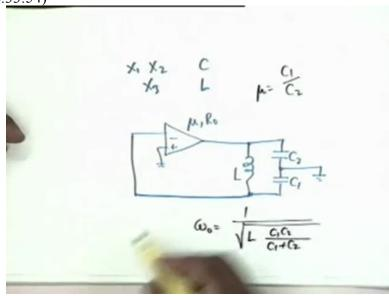
35:53If X1 and X2 are both capacitors and X3 is an inductor then the circuit becomes like this. Mew R0, we have an inductor here. Then two capacitors, this is C2 and this is C1. The middle point is grounded, these are connected. That is how it goes. Okay, now what would be the required mew?
