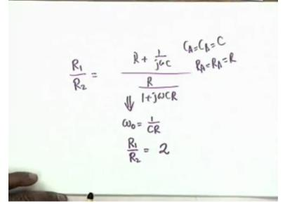
In the present case, if you find the condition for balance of the bridge, you will see that R1 by R2 is equal to R + 1 over J omega C divided by R by 1 + J omega CR and if you clear this, you will see exactly what we got for the condition of oscillation. Namely, you get a balance at the frequency omega 0 equal to 1 by CR and R1 by R2 has to be exactly equal to 2.
