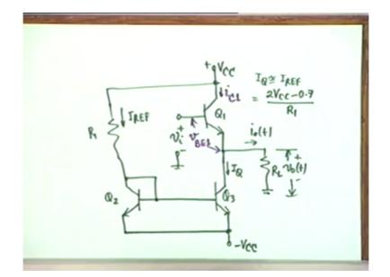
Then obviously the relationship is that V i is equal to v B E 1 plus V 0, agreed. Let us write this relationship that is worth 1000 words. This relationship as we will see V sub i is equal to v sub B E 1 plus V 0. If you recall the current versus base emitter voltage characteristics v B E 1 can be written in terms of I sub C 1 and the relationship is that this is V T log of the current I C 1.
