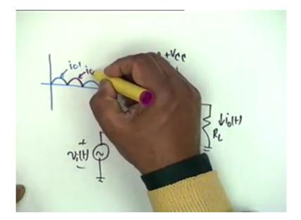
I C 2 are the negative half but the directions i c 2 comes like this so the load current is in the opposite direction. They help the load current to remain sinusoidal, okay. And I think that is all the picture that we need. Let us go into the calculation. Suppose the V 0 t is suppose V m sin omega t, alright? Then i 0 t would be equal to V m by R L sin omega t. It is a resistive load, agreed?
