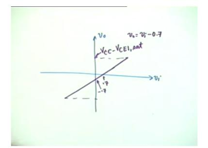
Let us look at the circuit. This voltage the maximum that can happen is in the positive side is plus V C C minus the voltage up here. On the other hand on the negative side the minimum value when V 0 is negative the minimum value that can occur is minus V C C plus V C E 3 sat. Is the point clear? Okay. So we have found out what the minimum is. Minus V C C plus V C E 3 sat. It is therefore important.
