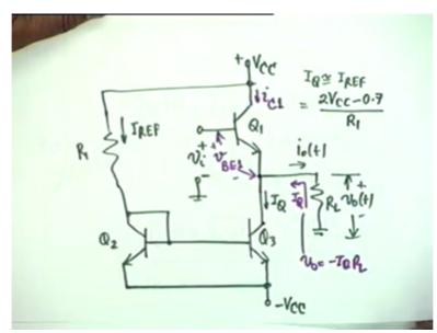
So P C 3 is V C C I Q. Now I have been able to get 3 V C C I Q by 2. What about the other one? Load power that is correct. What I missing is V C C I Q by 2 which I can write as V C C divided by root 2 multiplied by I Q divided by root 2. This is the RMS value of the load
