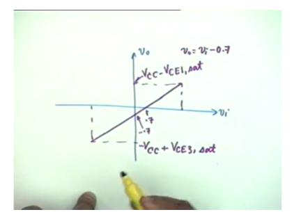
So you know the input voltages. The input voltage must not exceed these two values either on the positive side or on the negative side. You must be well within these limits. This figure only shows the limits, okay. You should not operate the transistor so that the peak swing goes here because then you are asking for distortion. You can as well go to class AB or class B amplifier, okay.
