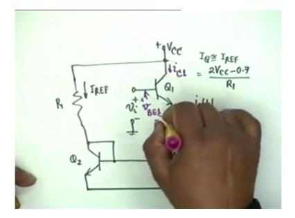
So physically much before this inequality starts affecting the circuit Q 1 shall be cut off which means that if we plot V 0 versus V i well we will have a plot like this. I am showing it a straight line. It will not be a straight line because there is a logarithm involved. It is a transcendental equation but it is very nearly a straight line. It is not exactly a straight line.
