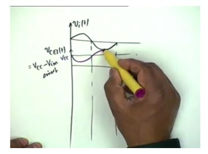
The maximum value here would be V C C plus V i m and the minimum value would be V C C minus V i m, is the point clear? Okay. If superimposed on V C C we are not assuming that V i m is equal to V C C that means we are assuming that because it is a class amplifier it is not driven to the maximum. We will see what happens when it is driven to the maximum.
