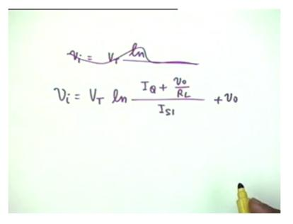
Now a problem arises when R L is small. When R L is small in the previous case we considered R L large so that the first term could be approximated by a constant, then the task was easy. When R L is small and these two terms are comparable to each other then the problem arises because when V i is negative, V 0 will also be negative. It is an emitter follower after all.
