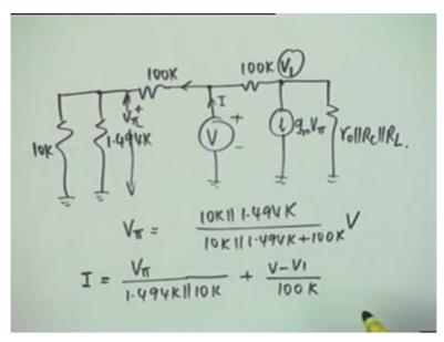
I now want to know what is V 1? Okay. We also see that this current is equal to g m V pie plus the current through r 0 parallel R C parallel R L so my third equation would be V minus V 1 divided by 100 K equals to g m V pie plus V 1 divided by r 0 parallel R C parallel R L. There are three equations now and the systematic way to proceed is to replace V pie. So we have one equation, second equation and this is the third equation.
