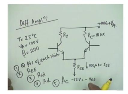
So the first thing that you should do, you should check the Q point that is find out I sub C and V C E. Now to find I sub C our procedure would be slightly different from what we were using earlier. You see what we do is first we write 10 volt equal to, do you know this current? How much? R C is given. R C is 100 K. This must be half of this, 50 microampere because beta is large, okay. So I know R C, I know 50, I know the current and therefore I know the drop here.
