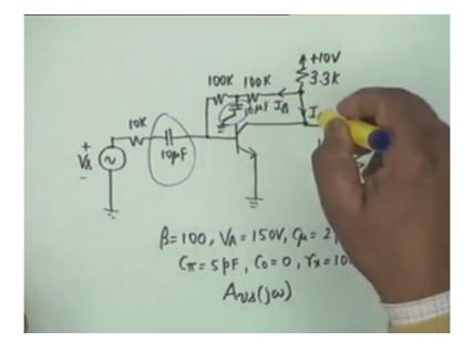
Therefore I expect that there shall be three critical frequencies omega L 1, omega L 2 and omega L 3. Let us call these capacitors are C 1, C 2, C 3. We therefore have three low critical frequencies omega L 1, omega L 2, omega L 3 corresponding to the three capacitances and there shall be two high frequency critical points corresponding to C pie plus C M, the miller capacitance. C pie plus C M will combine them.
