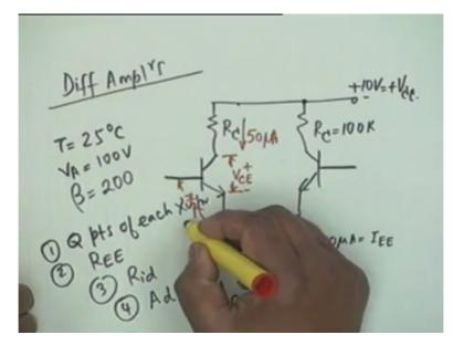
That makes a shortcut. I do not have to go through this. So my DC equation becomes 10 equals to 100 K multiplied by 50 microampere plus V C E then minus point 7 because I go from the emitter it to the base which gives me V C E as equal to 5 point 7 volt. Wonderful, so 5 point 7 volt and 50 microampere is the Q point of either transistor. Now to find out R E E. Yes?
