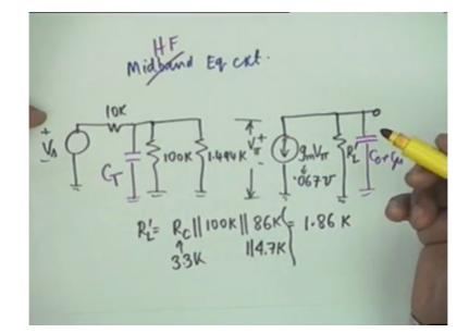
So after the approximation the method of time constants and the method of analysis are the same. As it is said the method of time constants has to be used when there are many capacitors. This is as good as analysis. It gives you same result as method of time constants and this is what was used to validate or give confidence regarding the method of time constant. That in simple case the results are identical. In complicated cases no sorry they are not identical, they differ, okay.
