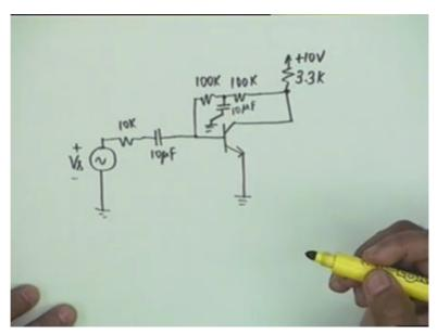
That is the current that flows through 3 point 3 K is I C plus I B and that I C flows here and I B flows here. It cannot flow this path therefore it comes to the base. We have done this kind of biasing. The only thing that was not done was this capacitor which is for obvious reasons
