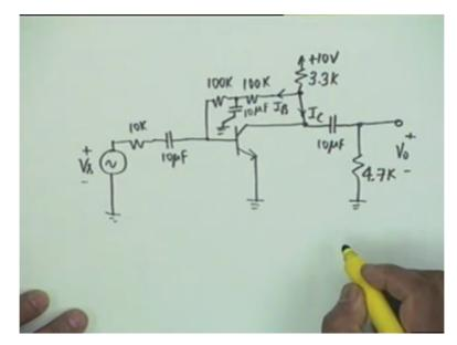
The transistor parameters are beta equal to 100. I do not want that murmur from there. Beta equal 100, V A equals 150 volt, C mu is 2 pars, C pie is 5 pars, C 0 is 0 no stray and r x equal to 100 ohms. Even though r x is given in most of the problems we conveniently ignore it because it increase is our problem of analysis, okay. The first thing we have to do is to find out A v s j omega.
