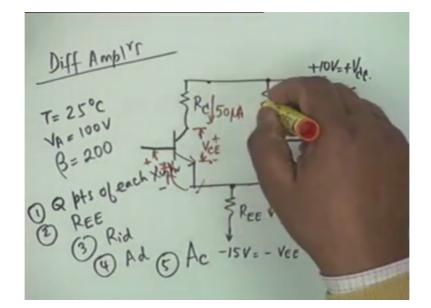
Any other question? Now to calculate R E E what we do is we come from here and go to the negative supply. We write a KVL. So what should I write? Point 7 plus R E E multiplied by 100 microampere then I have to go to ground via this supply minus 15, plus minus, plus minus, then minus plus therefore minus 15 which gives me R E E as equal to 143 K. Is this point clear?
