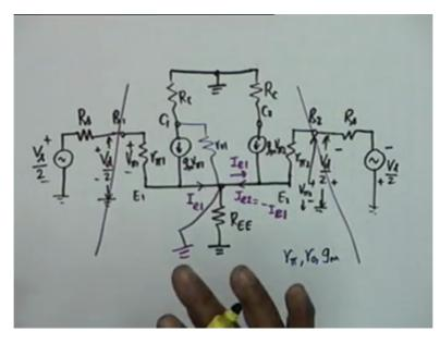
Now we can calculate the gain very simply. I can decouple this ground. I can only consider half of the circuit and this is called the half symmetry analysis. So what we do is we have an R s. We just take one of the transistors V s by 2 and then we have r pie 1 which now goes to ground. This is V pie 1 which is equal to V d by 2 with this polarity. Then we have g m V pie 1, 1 and 2 are the same.
