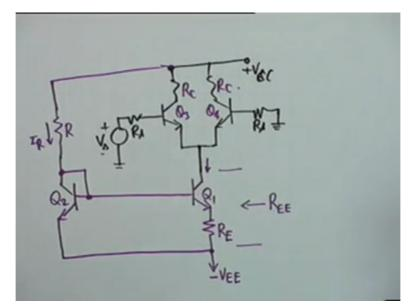
We have not increased V E E. We have kept V E E and V C C in the tolerable range. Effectively we want to increase R E E. If this transistor is ideal that is if its r 0 was infinity, if V sub a, the only voltage was infinite then obviously R E E would have been infinite, okay. But since there is an r 0 and V a is not infinity therefore R E E shall be a finite quantity but much larger than what we have physically connected here R E E.
