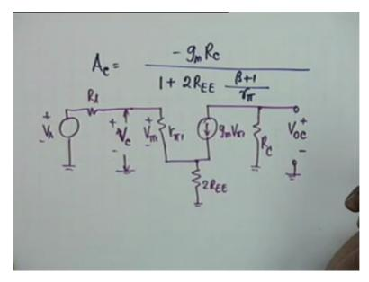
And if beta is much greater than 1 as have been assumed earlier this is simply beta by r pie and therefore g m and therefore this is approximately equal to minus g m R C divided by 1 plus twice g m R E E and initially twice g m R E E is much greater than 1 so the gain is simply minus R C divided by twice R E E. In condolence with what we have found out earlier. That in case of bypass emitter resistance the gain is controlled by the collector resistance and the emitter resistance.
