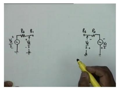
From base 1 if you look at the equivalent circuit we have an r pie 1. Base 1 to emitter is r pie 1 and base 2 to emitter is r pie 2 and the two voltages they are V pie 1 and V pie 2. I will run short of space, V pie 2, okay. Then the two emitters are connected together. This is E 1 E 2. E 1 and this is E 2.
