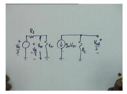
So what is the gain A sub d? It is V o d by 2 divided by V d by 2 and obviously this is equal to minus g m R C. The same result that we have derived from DC analysis, okay, the same result. We do not expect anything different. If it is different then we would have suspected our DC analysis. But it also shows two things that the output is an unbalanced output.
