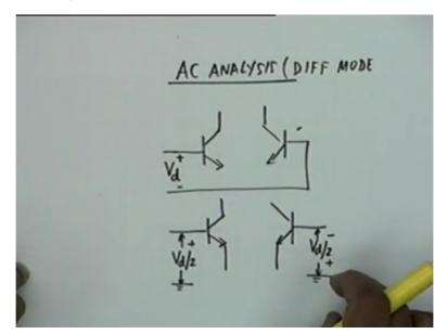
Let us look at the equivalent circuit. If I do that then let me view the signal also. Instead of V s let me view this as V s by 2 with this polarity and V s by 2 with this polarity plus, minus, okay, so that the total voltage applied is V s, the difference voltage. Now V d will be created
