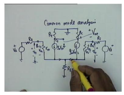
It is not equal and opposite to each other as in the differential mode which means that if this current is I e 1 then this current will be I e 1 plus I e 2 which are identical and therefore this will be twice I e 1 or I e 2. Yes?
