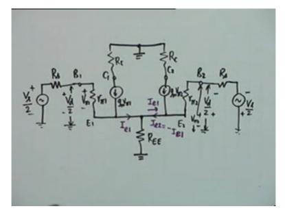
I e 1 comes here and goes away like this. No current flows through R E E which means that this point is virtually ground. This point is grounded and if that is so then the equivalent circuits simplifies greatly.
