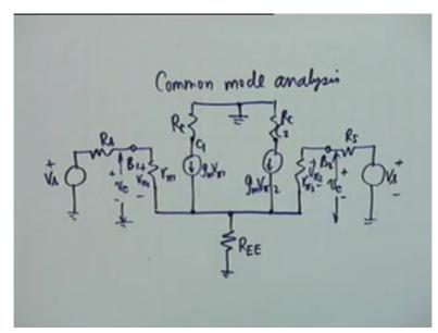
The only thing that we have changed is the sub sources are identical in the two sides and therefore the bass voltages are identical V c and V c. We want to see if there is an output from here to ground. Let us call this output as capital V small o small c, V o c output due to
