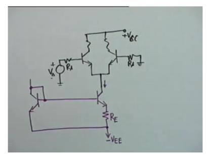
Instead of that R E E you see the complication. We have two transistors here and then I have to set up a reference current. How do I set this up? I had to have a resistance R here and this resistance is to be connected to plus V C C. So this is a differential amplifier R C, R C , this is a differential amplifier with R E E replaced by a current source, alright?
