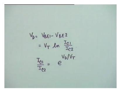
And therefore V D which = V BE1 – V BE2 shall be = V T log of I c1 divided by I c2, now we take the exponential on both sides that is I c1 divided by I c2 would be = e to the power V D by V T alright.
