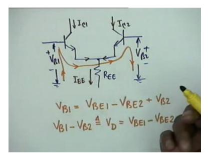
We go back to the same circuit we go back to the last one slide and we notice that this current is I sub c1 and this current is I sub c2 since we have ignored the base current, the same current must flow here and here I c2 so emitter current the current through R EE is I EE = I c1 + I c2
