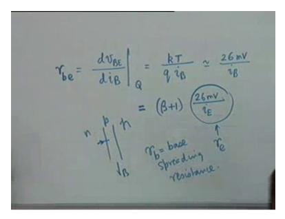
In the input junction if I take the ratio  $d \vee B \to d i B$  at the Q point the emitter base junction is a diode, and therefore this slope would be given by if you remember kT by q i B this resistance is the resistance appearing between base and emitter and therefore it is denoted by R B E base and emitter, not these symbols. This is small b small e which means that it is the incremental resistance okay, incremental resistance. Now this is kT by q and you know kT by q is
