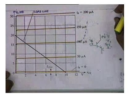
Obviously the active region is bounded by this line and this line okay. Is there a third bound. The question is, is there a third bound? Third bound comes because if you remember i C versus V C E while collector base junction is also a diode. A junction diode which is reverse biased. And V C E is reverse biased. And therefore I cannot continue to increase V C E without destroying the
