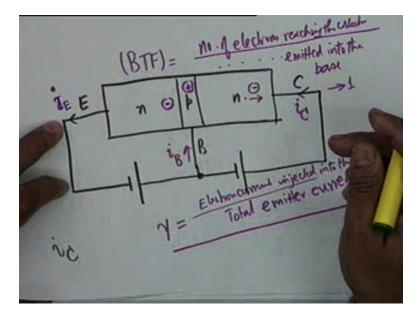
Now the question is this the only current that flows into the collector. Now you must realise that a collector base junction is a reverse biased junction and in reverse biased junction there is a current called the reverse saturation current and therefore the total collector current shall consist of not only the current due to the electrons emitted from the emitter but also the reverse saturation current.
