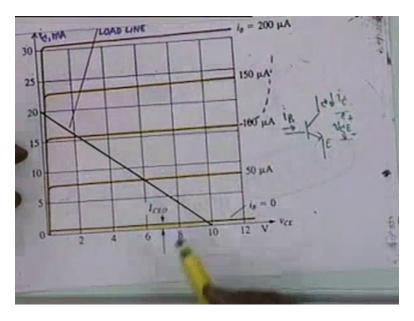
This is the point, when V C E is equal to 0. On the other hand when i C is equal to 0 V C E equal to V C C.
