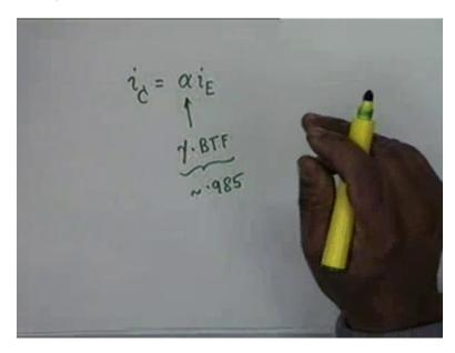
Let me change this slide, the collector current i C is a fraction of the emitter current Alpha i E where alpha is the product of, there are two reasons contributing to this constant alpha is a product of emitter efficiency and the base transport factor. And alpha in practice also is very close to unity because both these factors are close to unity and typical figure is 0.98 let say. 0.98 is not a very good transistors. It's more than 0.98 okay, may be 0.985 alright.
