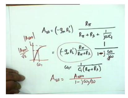
Therefore we can write A vs as = -g m R L prime then the potential division I can write as R Pi divided by R Pi + R s + 1 over j Omega C 1 agreed, and the effect of C 1 is obvious that = -g m R L prime multiplied by R Pi divided by R Pi + R s, I take R Pi + R s common then we have 1 divided by 1 + Omega 1 divided by j mega, where Omega 1 = 1 over C 1 multiplied by R Pi + R
