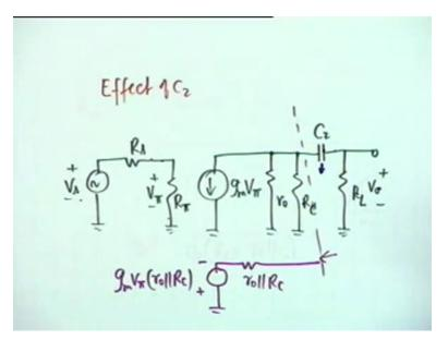
It is R L + the equivalent of this, is not this the Thevenin resistance that C 2 sees because this is a current generator and Thevenin resistance V s = 0 so V Pi = 0 so this current is 0 and therefore what you see is C 2 in parallel with R L + r 0 + R C okay.
