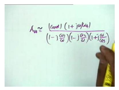
Now would you do not agree that our initial gas was A vs would be = some constant multiplied by 1 + j Omega by Omega 4 this was the initial gas, 1 - j Omega 1 by mega, 1 - j Omega 2 by Omega then 1 + j Omega by Omega 3 and remember we did not put this constant = A vs 0 why because it was not A vs 0, it was either A vs 01 or 02 depending on whether you consider Omega tends to 0 or Omega tends to infinity okay so this constant is not the mid band gain alright.
