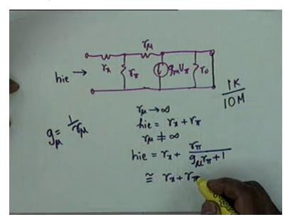
You calculate H I E from the hybrid pie equivalent circuit, R X, R pie, R mu, gm, V pie, R 0 okay. How do I calculate the H I E. H I E is the input impedance with the output, yes what we do to the output?
