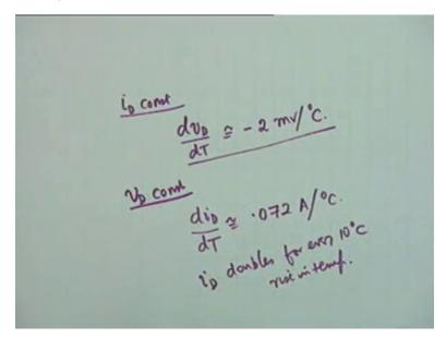
The characteristics of a diode are temperature dependent. Okay, this is one of the disadvantages of a diode. But it's also an advantage if you want make temperature compensation it's also an advantage. It is found that if i D constant that is if you drive the diode by current source a constant current source you inject a current i D then V D changes with temperature at the rate of
