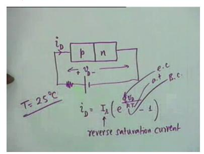
First we talk of a diode, as you know the semi-conductor diode contains basically, two types of semi-conducting materials brought in the neighbourhood of each other by metallurgical means okay. And 1 is a P type which is a preponderance of holes that is positive charged carriers. One is an N type which is a which is a preponderance of electrons which are the majority carriers. The P
