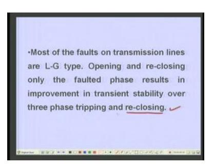
The reason is I have again let me reiterate most of the faults on transmission systems are line to ground faults opening and re-closing only the faulted phase results in improvement of transient stability over 3 phase tripping and re-closing. I think I will just mention about the steam turbine fast valving this is very promising technique for improving the stability of the system, we will discuss this remaining methods for enhancing transient stability in the next lecture.
