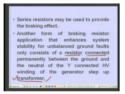
Now let us talk some few aspects about this. The series resistors may be used to provide the braking effect this point i will explain separately, another form of braking resister application that enhances system stability for enhanced for unbalanced ground faults only consist of resistor connected permanently between the ground and the neutral of the Y connected high voltage winding of the generator step up transformer.
