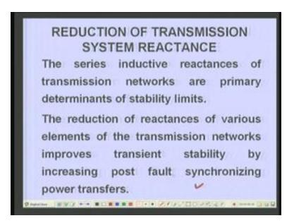
The reduction of transmission line or transmission system reactance we are talking of transmission system reactance. Now here the point is that series inductive reactance of transmission networks are primarily or primary determinants of stability limits the reduction of reactance is of various elements of transmission networks improves the transient stability by increasing post fault synchronizing power transfers right.
