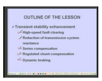
Under this category we will study importance of high speed fault clearing reduction of transmission system reactance under this category we will study how we can use series compensation to enhance the enhance the stability of the system by reducing the transmission line reactance then we shall also study about the affect of regulated shunt compensation on the stability of the system.
