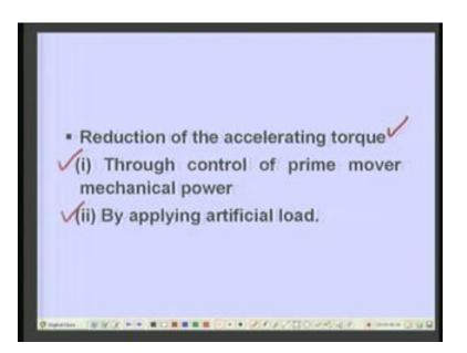
Another very important approach is reduction of accelerating torque that is we want to reduce the accelerating torque this can be reduced by by prime mover mechanical power control or through control of prime mover mechanical power you control this prime movers so that the mechanical power is is reduced when system is accelerating another is by applying artificial load.
