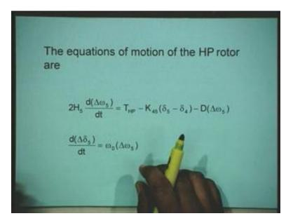
Now when we look at the high pressure turbine section then the there is no shaft on the left of the high pressure turbine section and therefore the net accelerating torque acting on the high pressure turbine rotor is  $T_{HP}$  the torque which is developed in the turbine section
