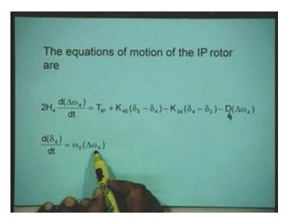
The equations of motion for  $I_P$  turbine section are writing in the same way as we have  $d_1$  for  $L_{PB}$  and  $L_PA$  sections that is 2 times  $H_4$  d by dt of delta omega 4 equal to  $T_{IP}$  plus  $K_{45}$  delta 5 minus delta 4 minus  $K_{34}$  into delta 4 minus delta 3 minus  $D_4$  delta omega 4 and d by dt of delta 4 equal to omega naught delta omega 4. Our next step is to write the equation for the last turbine section that is the high pressure turbine section.
