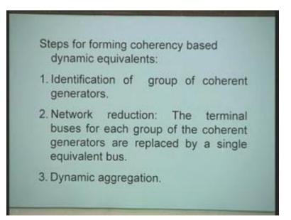
Now when we want to obtain the dynamic equivalents using coherency technique then they are 3 important steps which are involved, the first step is identification of group of coherent generators obviously that before I replace I before by replace the system by equivalent I should know that okay these machines are coherent, these machines are coherent, these machines are coherent, the groups have to be obtained, this is a first step and second step is called network reduction.
