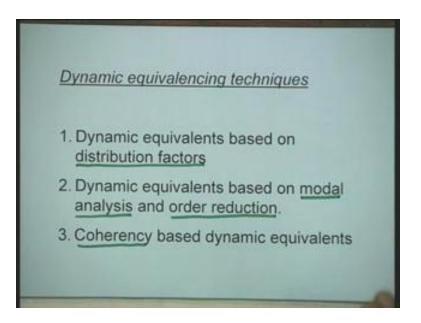
The techniques are classified under the these 3 categories that is the dynamic equivalencing techniques we can say or we can classify broadly in these three categories number one dynamic equivalents based on distribution factors, dynamic equivalents based on distribution factors, the second technique is based on a model analysis and order reduction model analysis and order
