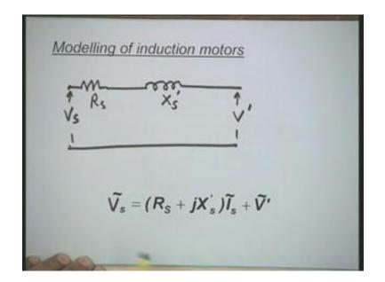
The stator of the synchronous generator can be simply represented by a model of this form. This is simple model which 1 can arrive at for the stator equation because the stator equations we are not considered the transform voltages right therefore this is a algebraic equation.
