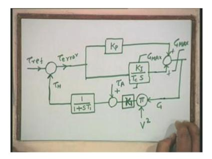
In any system, any system we want to regulate the temperature right then we start with the reference temperature let us call it tau reference and we want to know what is the actual temperature at any time T of the space okay. Now this this equation that is see this equation, this differential equation relates relates actually the time at a any time T with other parameters of the system this is simple differential equation, now this can be put in this form.
