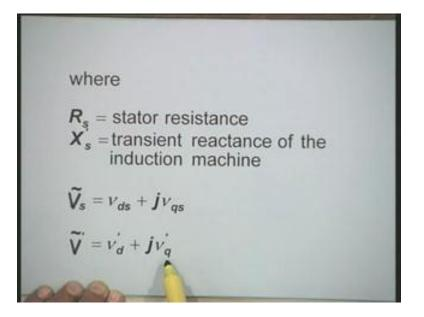
We can represent this voltage  $V_s$  bar as  $R_s$  plus j times X bar into  $I_s$  plus V prime this is an important voltage component okay when you represent these voltages in terms of D and Q axis components we can write down  $V_s$  equal to  $V_{ds}$  plus J times  $V_{dqs}$  V prime equal to  $V_d$  prime plus j times  $V_q$  prime.
