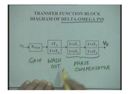
However, when we consider other excitation systems right then we have to account for the actual transfer function of the excitation system and further we can see 2 important points that the the the phase length which is produced depends upon the operating condition because it is function of the system constants and the constants are function of operating condition. Okay and it also depends upon the type of excitation system which we have considered right.
