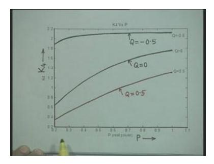
Now this graph shows the variation of constant  $K_4$  as function of real power output P for 3 different values of Q again that is Q equal to 0, Q equal to .5 and Q equal to minus .5 again you
