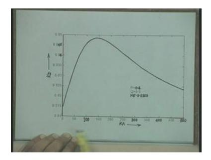
For the for the same operating condition the damping torque coefficient is plotted here and it is seen actually that the damping torque coefficient increases with increase in  $K_A$  and it becomes maximum for come value of  $K_A$  then it starts further decreasing. Now over this wide range of  $K_A$  that is um in this graph the  $K_A$  is varied from 0 to 500 right.
