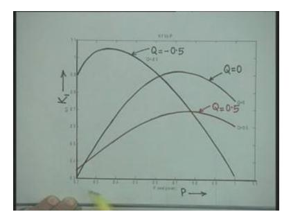
In this figure in this figure we have plotted the variation of constant  $K_1$  as a function of real power output P for 3 different values of reactive power output that is this graph shows this graph shows the variation of  $K_1$  variation of  $K_1$  for Q equal to 0 that is the reactive power output of the generator is 0 and we are varying the real power only okay.
