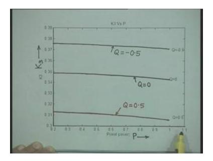
This constant  $K_3$  if you see that it is also affected by the reactive power output Q equal to 0 this is the graph Q equal to minus .5 this is the graph and Q equal to 0.5 this is the graph but for a given value of Q the variation in  $K_3$  as the value the value of P varies is very insignificant, okay this practically it is a flat curve.
