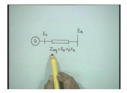
The system which we consider for small signal stability to start with is a machine infinite bus system where a synchronous generator is connected to a large system which can be characterized by a infinite bus, the equivalent circuit can be represented as generator the we represent the terminal voltage of the generator, the line is represented by an equivalent impedance Z equivalent equal to  $R_E$  plus j times  $X_E$  and connected to an infinite bus right.
