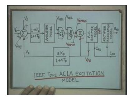
Now this block diagram gives you the complete model for the IEEE type AC1A excitation system, this is the IEEE type AC1A excitation system model. Now here you can start from the
