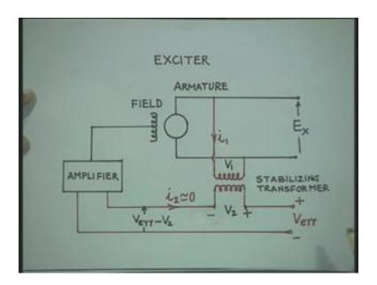
Therefore here, if I consider in general and exciter having its armature and field winding right the output of the exciter we represent as  $E_x$ . Now the this 1 simplest arrangement for stabilization which I have shown here is using a ah transformer that is you take a transformer and connect the primary of the transformer across the output of the exciter and the output of this transformer it is the secondary of this transformer is used to give a signal for stabilization.
