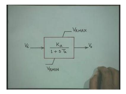
Now this amplifier will have the maximum and minimum limits that it respective what is the input signal coming the output will be limited to the maximum value because this  $V_{Rmax}$  and  $V_{Rmin}$ . For example, if you take the electronic amplifier okay there is always saturation and therefore the maximum value which is available will be determined by the characteristic of electronic amplifier.
