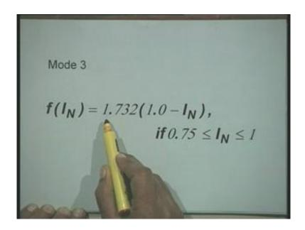
In the mode 3 operation this this function f  $I_N$  equal to 1.732 into 1 minus  $I_N$  where  $I_N$  is greater than .75 greater than equal to .75 and less than equal to 1 right. Now I have given you the expression for computing this quantity  $I_N$  earlier okay. Now the as I told you that in AC excitation systems we have different possible arrangements the model which I will be discussing here that is AC1A model that is IEEE type AC1A model right.
