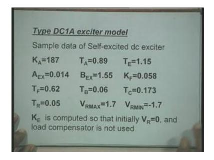
Now this transfer function model represents the both both self-excited, exciter self-excited DC exciter and separately excited DC exciter. The only difference is in the in the parameters of the model particular the K<sub>e</sub> right. Now here one interesting thing which is d1 here is that when we have a self-excited DC exciter, we set the parameters in such a fashion so that we get the desired
