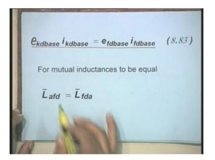
Now when you do this you will find this is very important relationship that is the base voltage in the direct axis amortisseur circuit multiplied by the base current in the direct axis amortisseur circuit this product must be equal to the the base voltage in the field circuit into base current in the field circuit, it is very simple that is the the base  $v_i$  in the amortisseur circuit should be equal to base  $v_i$  in the field circuit
