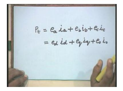
The terminal power  $P_t$  right which when we write down as  $e_a$  into  $i_a$  plus  $e_b$  into  $i_b$  plus  $e_c$  into  $i_c$  this is a terminal power okay. This  $P_t$  is average or instantaneous, instantaneous but what is average?
