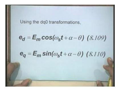
When you apply the dqo transformation you will get the d axis component  $e_d$  and q axis component  $e_q$  as  $E_m$  cos omega st plus alpha minus theta  $E_m$  sin omega st plus that is in fact when you apply this transformation right to arrive at this result we have to make use of many trigonometrical identities that is when you when you when you put these equations right  $e_a e_b$  and  $e_c$  this this column vector in that transformation matrix.
