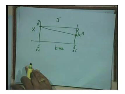
So, within that what I am specify, I am specifying the water availability, how much water you are entered to use. For example, storage is shown by X this is time, January this is the water storage X 0, this is the water storage in the January of 5; that means, this is the water, I can use provided there is no inflow, because inflow you have to consider that also; that is additional bonus water availability.
