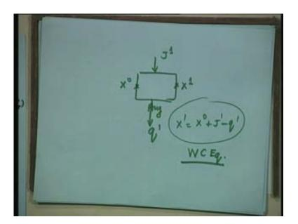
This is the reservoir, lets a month of August, in the beginning of August this is the water storage, at the end of August this is the water storage, during August this is the inflow and outflow is or discharge is q 1. So, X 1 is equal to X 0 plus input minus output, this is called Water Continuity Equation, Water Continuity Equation wish you must have done in control system plant equation
