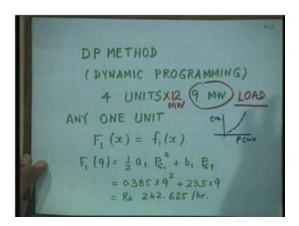
So, similarly, here I take an example of 4 units each unit is of 12 mega watt capacity, each unit is of 12 mega watt capacity and I have a load of 9 mega watt. My job is to satisfy load of 9 mega watt. This is the small township village, may be of 100 people and load is in 9 mega watt and 4 units of small. Now we are going was smaller units as I told you, dispatch system you know, distributed system.
