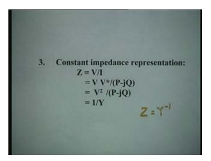
And the third is constant impedance Representation or there are inverse of each other Z is equal to one over y or if it is matrix or Z is equal to y inverse v by I we have just found out value of I V square by P minus j Q one over Y, so this is constant the load of 5
