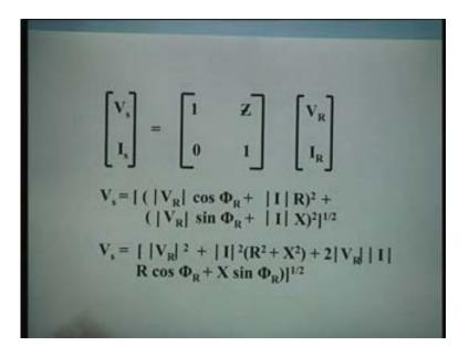
Let us write the equation these are the equations V s I S 1 0 1 V R I R, I can write V s in this particular form V R cosine phi R plus I R whole square plus V R sin phi R plus I X whole square, you may ask me from where you got this equation.
