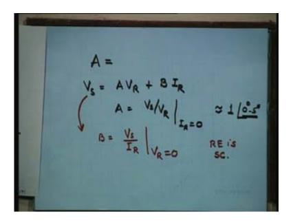
A can be find out, which is as simple as that, that is write the whole equation V s is equal to A V R plus B I R. So, A will be equal to V s upon V R with I R is equal to 0, where you say I R is equal to 0 is what? hm. Open circuit. Open circuit, absolutely, Very good, the receiving end is open circuit.
