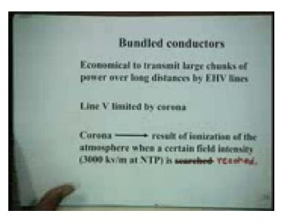
So, bundle conductor is entirely different concept then ACSR conductor, it is economical to transmit large chunks of power over long distances by EHV lines, this we are telling you from very beginning, that is why there is a need of transformer, because generation is always at lower voltage up to 25 k v you cannot to beyond; why, there are cooling problem, there are insulation problems, safety problem, but the transmission is always cheaper, convenient, economical on EHP or UHP line.
