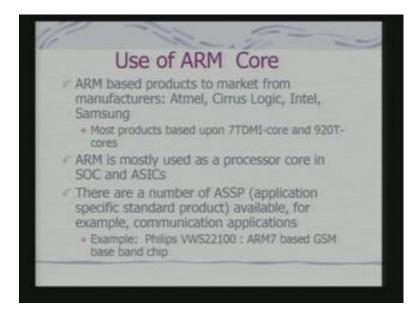
So, what we have got is variety of features in the ARM core, which enables it is use for an number of application. In fact, ARM core or ARM processor architecture has been licensed to a number of users. And they have used Atmel, Cirrus logic, Intel, Samsung there are may products out of each. And ARM is mostly used as a processor core in SOC and ASICs as well.
