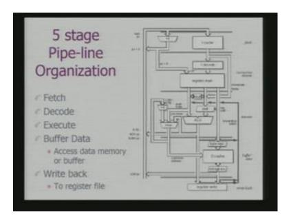
It implements not a 3 stage, but 5 stage pipeline and this changes what implemented to achieve a kind of a CPI of the order 1.5. And to improve the maximum clock frequency. This 5 stage pipeline has got the following stages, fetch, decode, execute, buffer data, write back. In fact, these are the two modes, which are last to other two modes which are not their originally.
