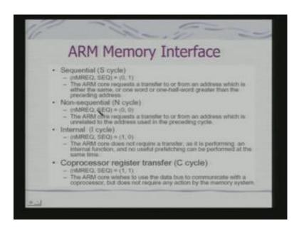
The ARM memory interface has got I have already shown you the cycles. And this is exactly the definition of the details of the cycles. So, it says the ARM code now request the transfer to or from an address, which is at the same or one word or one half word greater than the preceding address. This is exactly the meaning of sequential access. This is non-sequential access, where it is not related to the previous address. And this is corresponding to coprocessor register transfer.
