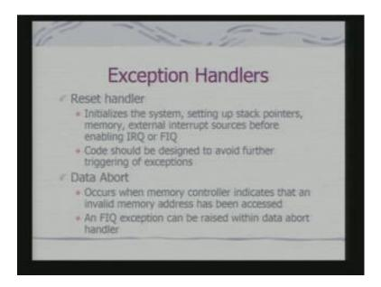
So, how do you designed exception handlers. Typically reset handler initialize the system, it is sets up stack pointers, memory, external interrupts sources, if you needs to initialize the peripherals before it enables IRQ or FIQ. Because, you would not like to have ((Refer Time: 09:05)) interrupts before the external devices have been initialized.
