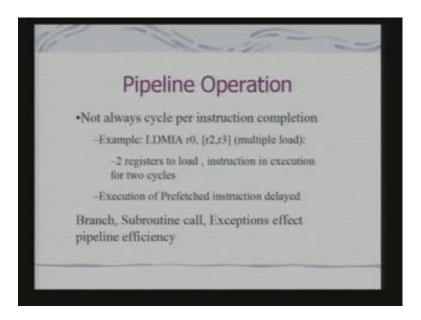
So, there are, but one thing with ARM instruction set is that, all instructions are not necessarily single cycle instructions. The typical example is load multiple byte or load multiple or stored multiple instructions. So, these the multiple load. So, it has got 2 registers to load and so the instruction has to be in execution for two cycles.
