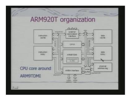
This ARM920T is basically using this as a processor core, this is as a CPU core. This is what you get the complete processor core. So, you have got an instruction cache A, instruction MMU this is the memory management unit for your instruction memory. This is than the memory management unit for your data memory. So, you got to a two MMU's.
