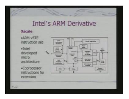
And Intel has made one such enhancement, which is called X scale architecture, which is built around ARM 5TE extension. And this architecture is different, Intel develop its own micro architecture and coprocessor extensions.
