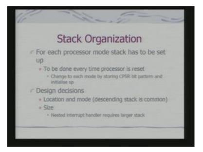
Now obviously, for doing all these exception handling, you have understood always the stack organization becomes critical. Because, for each processor mode I have got a stack pointer and each processor mode has got a different stack therefore. So, I need to set up this stack in the beginning itself. So, every time this stack this is not a single stack. So, what I shall have? I shall have a stack in the memory.
