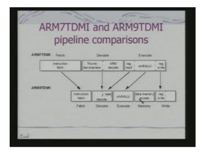
And this is a kind of a comparison between ARM 7 and ARM 9 pipelines. ARM 7 had a 3 stage ARM 9 has got a 5 stage. In fact, what we are showing here is that, thumb decompress and ARM decode is actually everything put together to a decode. Because ,this is TDMI; that means, I have got a thumb mode as well takes place here.
