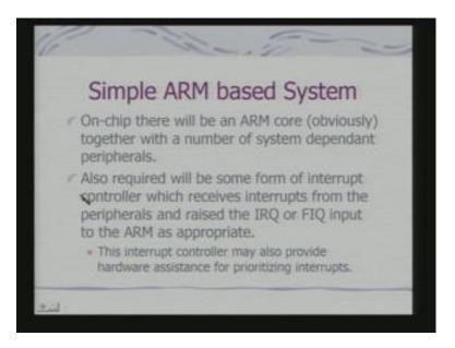
So, a simple AMBA system what should be there. On-chip, there will be an ARM core with a number of system dependant peripherals. Also required will be some form of interrupt controller, which receives interrupts from the peripherals. And raised IRQ or FIQ input to the ARM as appropriate. So, an interrupt controller may also provide the hardware assistance for prioritizing the interrupts.
