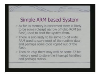
So, it is becomes the part of the hardware as for as memory is concerned there is likely to be some narrow off-chip ROM or flash, which will be used to boot the system from. Because, during develop in face, you will be using the code from the core system maybe to test on the chip using your JTAG port. But, actually your code has to going to the flash or a EPROM in and for an embedded system.
