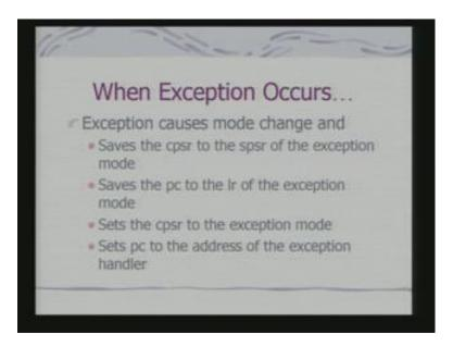
So, along with mode change what will happens? The core saves CPSR, that is Current Status Register to the SPSR of the exception mode that is saved a registers. There is save PC to the link register of the exception mode. Sets the CPSR of the exception mode and then, set PC to the address of the exception handler. In fact, all of this exceptions are associate with the vector. That is a memory address at which the exception handler is expected to be located.
