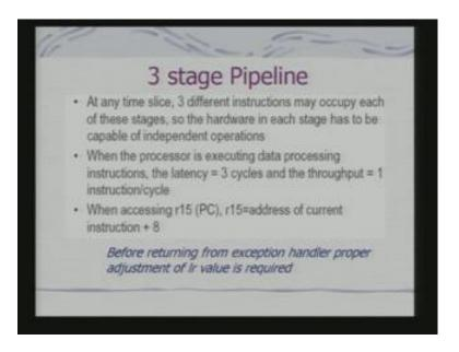
At any time slice therefore, 3 different instruction may occupy each of this stages. And when the processor is executing data processing instruction, the latency is 3 cycles and throughput is one instruction per cycle. I hope you understood why latency is 3. And when accessing r15. R15 is address of current instruction plus 8, this is the key point.
