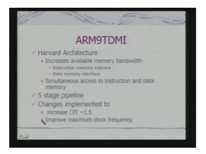
Next, we look at ARM 9 which is an enhancement over ARM 7. Now, ARM 7 was a Von Neumann architecture, this is Harvard architecture. Obviously, the Harvard architecture ensures increased data transferring. Because, you have got a separate instruction memory interface and a separate data memory interface. So obviously, the memory bandwidth is more.
