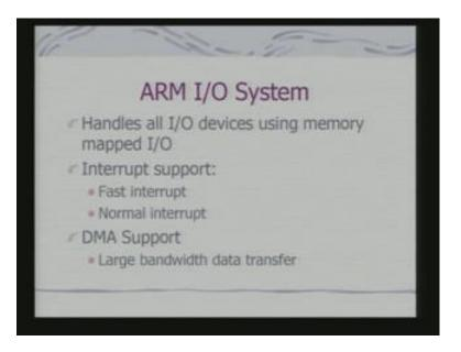
In fact, I/O system, that I/O devices they are primarily interface through this kind of interrupts. So, I have first interrupt in normal interrupt that we are already discussed. And there used for interrupt driven I/O processing and all I/O devices at typically located in the memory map of ARM.
