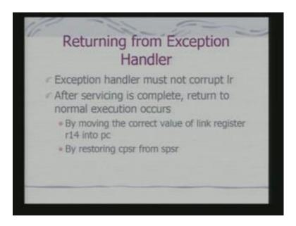
So, how do you return from exception handler, it can be using any instruction for that matter, which will restore your PC to the corrected value of the link register. And what is important is that, the exception handler must prevent corruption of the link register value, which gets loaded when more switch takes place. This is very, very important.
