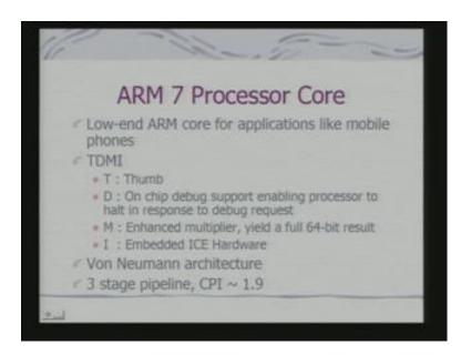
We have look at the data path of ARM 7. But, not only the data path there are other; obviously, the hardware components, inside the ARM 7 processor. In fact, ARM 7 is the
