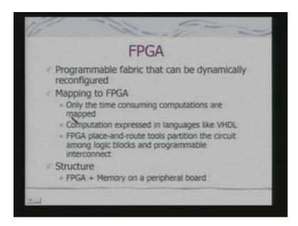
Now, what are these FPGAs really if you are trying to design a function, we should know what are these FPGAs, in fact FPGAs are in a way a programmable fabric that can be dynamically reconfigured. In fact, this point we have looked at when you looked at reconfigurable SOCs. So, basic job now turns out to be mapping of your task to FPGA. Typically, only the time consuming computations are mapped, that computations which are basically bottle neck.
