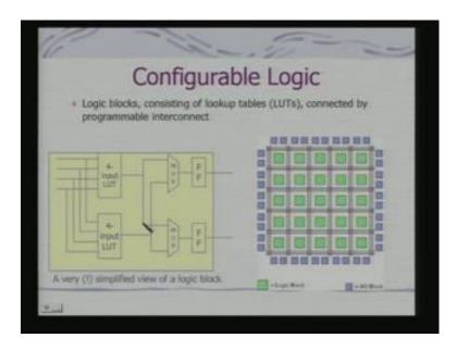
So, what are really FPGAs, FPGAs we said is the configurable logic and here we are showing a very simple example. In fact, this is a basic logic block, you have got a four input LUTs, so it is a kind of a combinational circuits, this is another 4 input LUT. So, depending on the four inputs you can synthesis any 4 input functions the basic idea is that and this is the multiplexer, depending on control inputs you can choose the functions from this two blocks and these are the flip flops.
