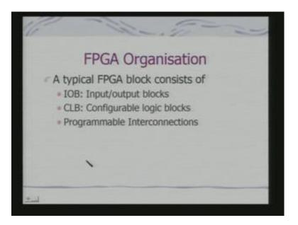
So, typically therefore an FPGA consists of following blocks, what we call is IOB that is input output blocks. Then you have got configurable logic blocks, these are the basic units to which your functions are mapped and then you have got programmable interconnections.
