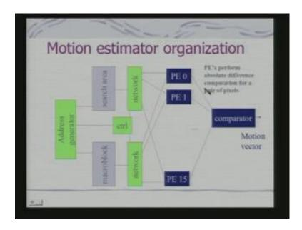
So, this is one of the possible architecture, if you see here this is the memory macro block and the search area this contains the data, this is the basic address generator and this PEs are implemented on the FPGA block. Each PE does what, perform absolute difference computation for a pair of pixels and your comparator takes the data from PE integrates it together and produces the motion vector corresponding to the best value.
