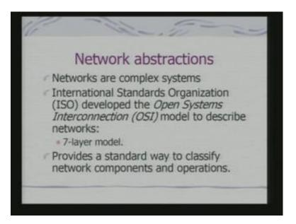
Now, networks; obviously, of therefore, complex systems. So, we need some mechanism or abstraction the most common abstraction is the 1 which was propose by ISO or known as open source interconnections model or OSI model and that is the seven layer model. And it provides a standard way to classify network components and operations.
