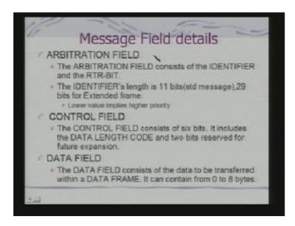
So, arbitration field actually consist of what is called the identifier and RTR bit. In fact, RTR bit indicate whether it is a data request frame or a actually a data frame the
