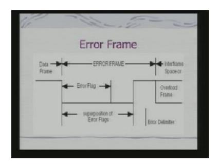
So, the error frame look something like this. So, here are the error flag and this is the error flag which is transmitted once the error is detected by the corresponding transmitter are the basic.
