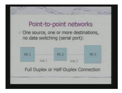
So, the simplest network that we can have is a point to point networks there is 1 source and 1 destination and there is no data switching. So, if you a built a building a network over the serial port between the PEs we shall have this a point to point network connection it can be a full duplex or half duplex communication.
