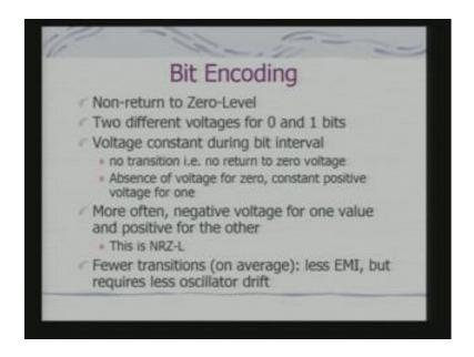
Next comes the bits encoding; at the bit level how the bit information is encoded typically what is used is non return to zero level this is the standard way of sending digital data non return to zero level. There are 2 different voltages for zero and 1 and voltage is constant during bit interval. So, no transition si that is no return to zero voltage
