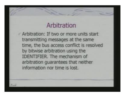
Two or more units start transmitting message of the same time and it is a resolved by using the identifier priority the mechanism of arbitration guarantees that the neither information nor time is strictly lost. So, that arbitration mechanism is an interesting part of CAN and we shall discuss it later on first let us start looking at the physical layer.
