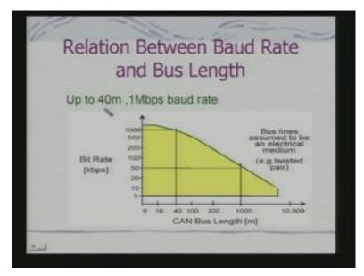
So, up to forty meters it can work at typically 1 Mbps as the baud rate. So, this is typically the characteristics of a CAN. So, 40 meters what you can realize that if you are looking that an appliances like car are any such this 40 meter is good enough. And so, I can have a high speed data transfer inside an application like car.
