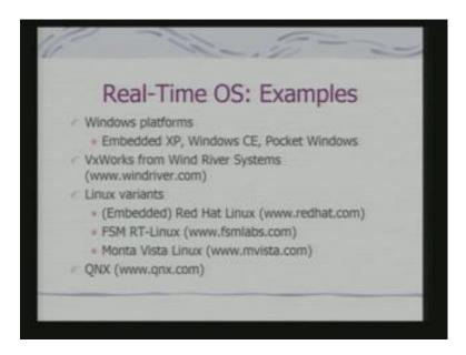
There are number of such examples which are available and today being used windows platform this are primarily source from Microsoft targeted for handle devices then VxWorks from Wind River system possible. The most well known commercial operating system used in embedded appliances. There are variety of Linux variants therefore, Linux is now is turning out to be the most popular in fact, on an upward swim for its application in embedded domain.
