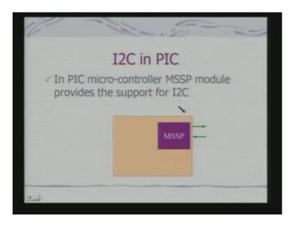
In variety of microcontrollers and in PIC family as well typically this MSSP module which is their in PIC provides the support for I2C.
