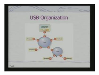
So, you have a host device. So, do a host device you can connect the hub and your peripherals gets connected to the hub otherwise you connect a single peripheral with the host device so, I can build now a tree. So, if I connect at one port another hub, I can connect more peripheral to this and that is why this is called a bus; that means, there can be multiple devices hanging from one link.
