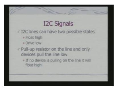
So, I2C lines can have 2 possible states what we say a float high and drive low and pull up resistor on the line are connected and only devices pull the line low. So, if no device is pulling on the line it will float high; that means, by default the I2C signals will be always high.
