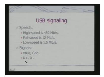
Typical speed is a high speed bus between. In fact, if it is a high speed its 480. In fact, 12 Mb it can walk to the lower speed is 1.5 Mb. Signals are basically Vbus that is a this is basically the power signal in the ground and the other signal is basically D plus and D minus is the differential levels for communicating the data.
