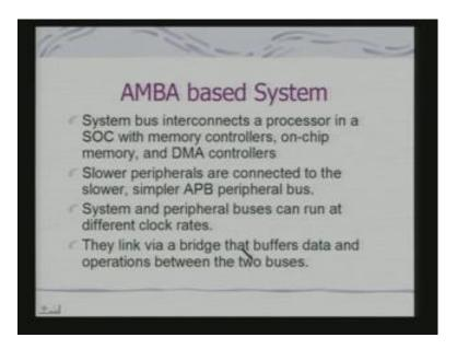
So, system bus interconnects a processor in an SOC with memory controllers on chip memory and typically DMA controllers. Slower peripherals are connected to the slower and simpler APB peripheral bus and this system and peripheral bus; obviously, it is expect to run at different clock rates and they link via bridge that buffers data and operations between the two buses. Why it needs to buffer data? Because, there is a mismatch in the speed between the 2 buses.
