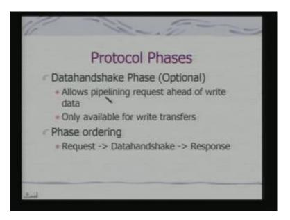
Similarly, there is a Datahandshake Phase which is a part optional a part of your protocol phases. So, what we says that allows pipelining request ahead of write data and only available for typically write transfers. So, the Phase ordering typically for a transaction would be request at Datahandshake followed by response.
