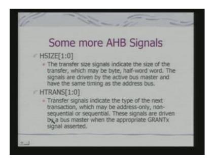
Some more AHB signals are size. In fact, this size we have already seen in the context of ARM signals memory interface signals also an it is consistent in that context and edge trans. This transfer signals indicate the type of next transaction which may be address only non sequential or sequential. These signals are driven by a bus master when appropriate GRANTx signal is asserted. So, that to prepare the devices to expect what kind of transactions would ((refer time: 26:36)) next.
