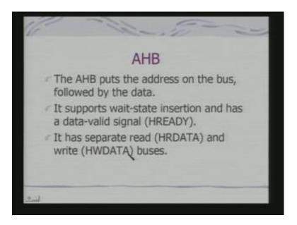
So, how it works? AHB puts the address on the bus followed by the data if it is a write. So, the master provides the data it is supports wait state insertion and uses a data valid signal which is called HREADY which is just take a ready or a wait signal that you fine with ARM.
