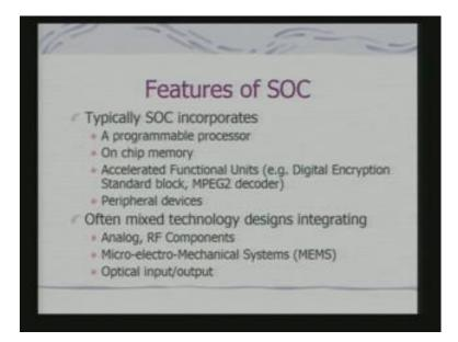
What does the features of this SOC? Typically, our SOC incorporates a programmable processor on chip memory. Some additional functional units, which are more application
