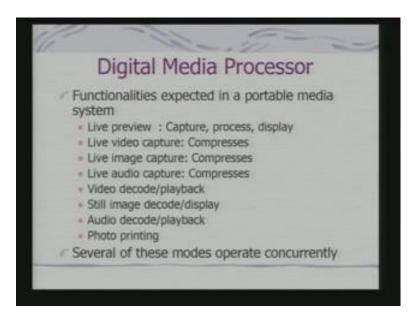
In fact, the another example, towards this direction is digital media processor, which are called portable digital media processors for providing all this services in a standalone modes. So, what we say that, you have device a chip, which can support video. As well as image capture, audio capture, video playback, audio playback, printing interfaces. So, it is just not a camera, just think that if you have such a SOC, you can be a devices which will not be just a camera.
