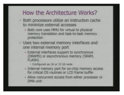
Now, how this architecture really works. Both processors, utilize an instruction cache to minimize external accesses. That is what we have already seen, in the architecture diagram. And they both use MMU, memory management unit, for virtual to physical memory translation and task-to-task memory production. Because, there tasks these processors will have distinct task. And there task need to be protected against violations of access.
