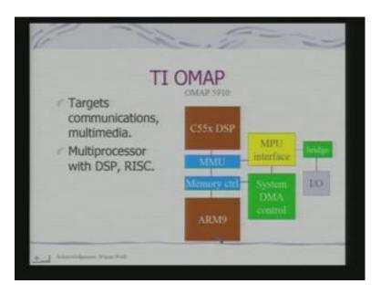
TI OMAP has got C55x DSP, we have studied that already as well as ARM9, these two. And there are variants, this is we are looking at one particular OMAP. And they have been used together for multimedia, as well as... In fact, handled portable communication terminal applications.
