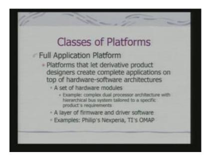
There are different classes of platforms full application platform. Platforms that let derivate product designers create complete applications on top of hardware-software architectures, that I was talking about. So, it can come with the set of hardware modules. It maybe a complex dual processor architecture, with some kind of an hierarchical bus system tailored to a specific product's requirements. And use that hardware, a layer or firmware and driver software as provided.
