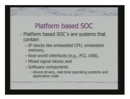
So, what we are talking about, a platform consist of IP blocks. Like embedded CPU, embedded memory. And when it comes in a form of a hardware, you may not know the details of it. But, you can also use the layers and the features provided on the platform, for developing the application. So, a platform can come with an embedded CPU, embedded memory, real word interfaces, mixed signal blocks and software components the tools to use all this elements, which has been put into the platform.
