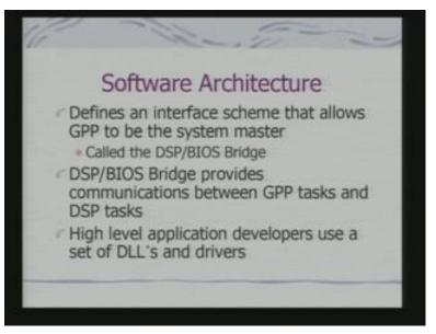
So, what is your software architecture this becomes a key thing, because somebody, some manufacturer can design a complex hardware SOC. But, if the proper software interface or the software architecture is not defined. Then, using this SOC is becomes extremely difficult. And that is precisely the reason, the point I was making all through that platforms essentially mean, packaging of both hardware and software together.
