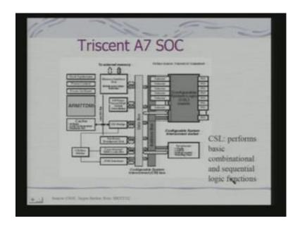
A simple example is this Triscent A7 SOC, which is again using your ARM7. That we are already studied and this is your configuration system logic block. And these are units which perform basic combinational and sequential logic functions. So, collection of gates, they can be configured to realize different function. And I can use a set of search gate to realize these functions together.
