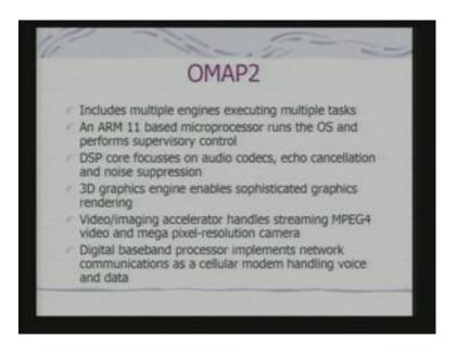
Now, we have got multiple engines, executing multiple tasks integrated on the same chip, that is What is OMAP 2. Here, you have ARM11 based microprocessor, which is advanced version from ARM9. DSP core focuses on audio codes, echo cancellation and noise suppression. These are primarily important for caring out telephonic conversation. There is on top of that, a 3D graphic engine which is again basically a processor to enables sophisticated graphics rendering.
