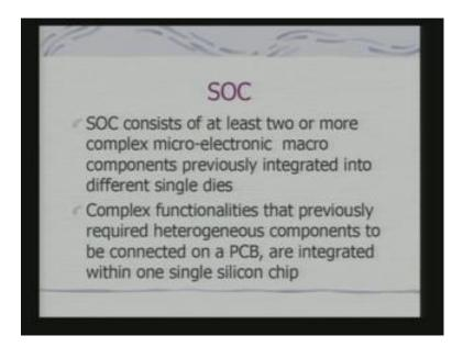
SOC are system on chip, consists of at least two or more complex. Microelectronic, macro components, which are being previously integrated into different single dies, in individual form. Complex functionalities, that previously required using heterogeneous components; and designing a PCB. And interconnecting them on a PCB. And now being integrated, within one single silicon chip.
