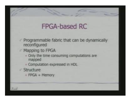
So, what we have got now, what are called FPGA based RC, that is programmable fabric, that can be dynamically reconfigured. Any of two mapped therefore, this code to FPGA, link on figure the FPGA. And then, do the computation. So, you have got a programmability not in just software, but as well in hardware.
