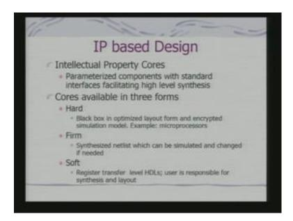
And what you get is intellectual property cores, as the basic components of such a design. In fact, when we are talking about ARM processor; and we refer to as ARM core. So, ARM core becomes an intellectual property core. And what is essentially in that context, that interface of that reusable component has to be known, and known to whom, known to an application developer, who is designing the system on-chip. Now, this course are available in a variety of form for this purpose.
