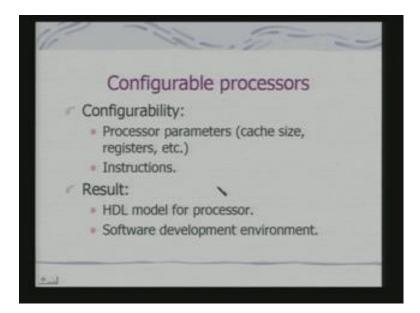
The other end is also configurable processors. The previous example what we said we have a processor as well as FPGA. We can now configure this FPGA or this ALU's depending on the applications. Here, we are looking at configurable processors. So, processors can source can be configured before you actually go into a design. So, processor, parameters, registers etcetera can be configure.
