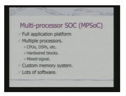
This multiprocessors SOC or MPSoC, they are typically full application platforms. In fact, other way round majority of your full application platforms are nothing but, multiprocessor SOC. So, they have got a CPU and a DSP. These are many minimum and common requirement. Some of the special hardware blocks, the hardware blocks designed from special purpose functions. And there will be mixed signal elements, that means you are for analog interfacing.
