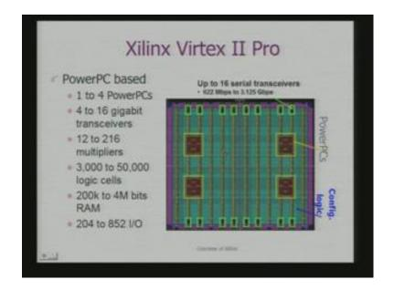
This is an example of this kind of programmable platform that I was talking about Xilinx Virtex II Pro. It has got 4 power PC processor cores sitting on the same SOC along with the FPGA logic. To add on the hardware and it has got serial transceivers to transfer the data.
