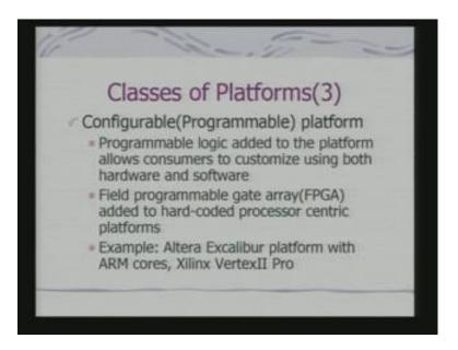
Then we can have configurable platforms. Here, the programmable logic is added to the platform, which allows consumers to customize using both hardware and software. So, you have got field programmable gate array, added to hard-coded processor centric platforms. So, when you talked about processor centric platform, it was primarily the processor. And some additional components, with a software services bundled with that processors centric platform.
