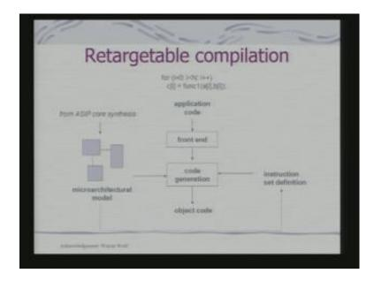
How will a software tool behave? Will you design a software tool for each an every variant of the processor that you are producing. So, you have concept of what is call retargetable compilation. So, that retargetable compilation takes as input the architectural modal, as well as the language specification and that is used in the code generation block.
