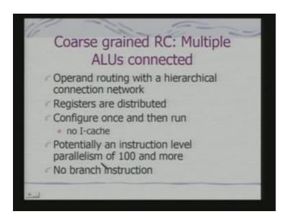
Then we can have coarse-grained re-configurability we have got simple logic gates putting together logic gates to realize simple logic functions. From there you can have a set of ALU's and you know configure this ALU's and the set of registers to do some tasks. So, it becomes an example of a coarse-grained re-configurability.
