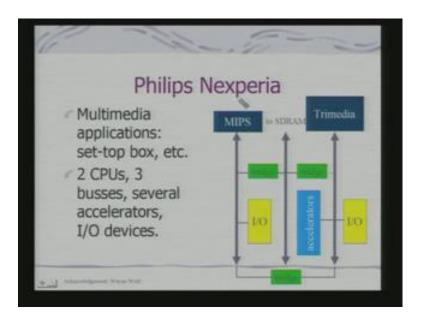
So, here we have talked about Trimedia CPU Philips and MIPS processor, which is an example of a RISC processor. These two code set together and you have got other accelerators, which are meant for accelerating some special functions. And these are the individual buses and buses to SDRAM and the bridge, between the buses of the individual processors. So, this is a kind of a multiple processor system.
