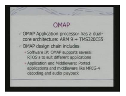
OMAP application processor, we have already seen has a dual core architecture. ARM9, as well as C55 DSP. And it is design chain includes software IP, there is OMAP supports several real-time OS's, to suit different applications. So, you can use that OS's to program, these SOC for application development, also application and middleware. There are ported applications and middleware, like MPEG-4 decoding audio playback. MPEG-4 is a video decoding, a video standard.
