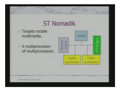
This is an example from ST. Now, this is very interesting, because it just not a target mobile multimedia but, it is not just two processor, it is a multiprocessors of multiprocessors. So, you can see the complexity to which the design can go up, when an SOC is being designed for applications. So, here the audio accelerator and video accelerators, are collection of heterogeneous multiprocessors. And they are actually used along with the ARM9 core to provide your platform.
