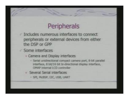
A number of peripherals can be interfaced, a number of interfaces are supported. We shall look at some of this interfaces because, they are interesting, in terms of the target applications. It provides camera and display interfaces, because if I am targeting for this kind of embedded portable terminals. Then, they will typically have a camera connected to it. And so that camera interface, forms a part or an integral component of this SOC.
