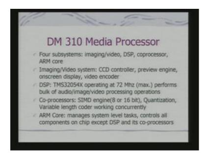
And taking this into account, there is a DM310 media processor, which is again an SOC a multiprocessor SOC. And it has got four subsystems, imaging and video, DSP a set of coprocessor, as well as ARM core. And in fact, that ARM core is being used in a very extensive fashion. So, you have this imagine and video system, has got a CCD controller. I hope you remember that, we had talked about CCD as a basic imagine sensor.
