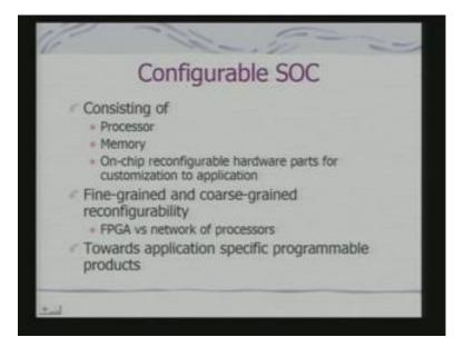
What are reconfigurable platforms, reconfigurable SOC is, typically consist of processor memory as well as on-chip reconfigurable hardware parts, for customization to application. These could be fine-grained or coarse-grained, when it is a fine-grained you have got FPGS. The excrement of the coarse-grained, there can be a network of processors, a multiple processor and this processors can be configured for your work.
