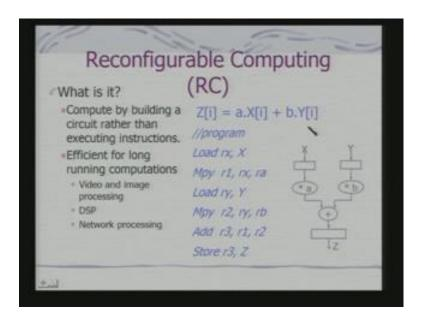
So, what we say, that compute by building a circuit, rather than executing instructions. Take for example, a simple multiplication here. I am multiplying the two elements by constant a and b. And I am trying to compute the result. Now, what is the interesting here is, this is the set of assembly language instruction. So, it is a multiply load, you can understand this will be used for computing this function.
