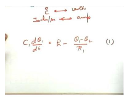
You see that C d theta 1 by dt let me call it C 1 dt is equal to h minus theta 1 minus theta 2 divided by R 1 where let me call C 1 as the thermal capacitance of the system and R 1 as thermal resistance of the system and now onwards if you understand this point I need not take up these variables in terms of mass, specific heat, film coefficient, area and all that. I assume
