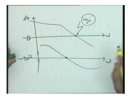
Now look at the phase margin. So, at this particular point if I measure the angle with respect to minus 180 degrees this is your phase margin. In this particular case the phase margin is negative it means whatever plot I have made over here without any transfer function in front of me has turned out to be the open-loop plot for a closed-loop system which will be unstable because the phase margin is negative in this particular case so the system will be unstable.
