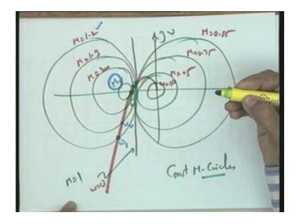
Therefore, I find that as I travel along this particular Nyquist plot from omega is equal to 0 to infinity the magnitude of M is increasing, becomes maximum and then starts decreasing and therefore from these particular circles I can make a sketch of this type which is the closed-loop response of the system.
