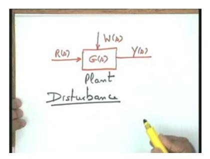
G(s) this is the input R(s), let me call this as the input you manipulate and this is the input here W(s), W letter you recall was used for disturbance so capital W(s) will be the disturbance in Laplace domain and this is your Y(s). This in fact should be the input output configuration where G(s) is a plant model because we know that these are the two types of inputs the plant will be subjected to.
