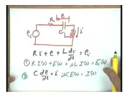
The manipulation in this particular case gives me G(s). Please help me, what is the output variable in this particular case? Output variable is Y(s) which you have to define divided by the input variable E i(s). Y(s) or y(t) is an attribute you are interested in. And in the last example y(t) was taken to be voltage across the inductor.
