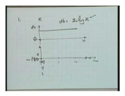
Therefore, coming back to the first building block I find that the first building block is simple constant k and it does not create any problem; a magnitude line horizontal and a zero phase line. Go to the second building block please; the second building block let me take 1 over j omega though I told you in general it is j omega plus minus N. Let me get started with only 1 over j omega and then I will see what happens if the value if the type of the system increases from 1 to 2 and so on.
