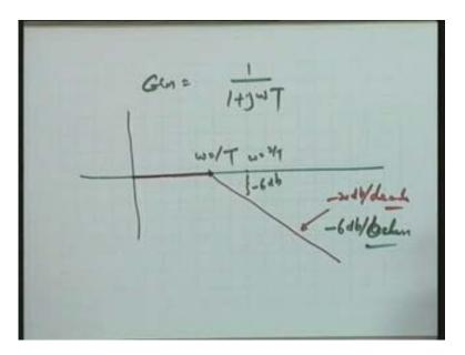
This is your corner frequency and this is called asymptotic Bode plot please. Now, from the asymptotic Bode plot the actual plot will come in the following way; just mark a point 3db down, take one octave below, mark a point 1db down, take one octave above mark a point 1db down and join these making asymptotic to the 0db line and asymptotic to minus 20dbs per decade line this becomes your accurate Bode plot without any calculations.
