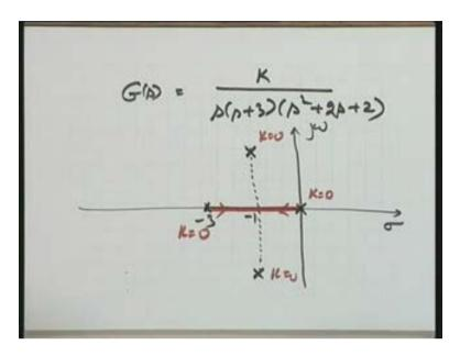
We will make the calculations later and for that I make the pole-zero diagram so that it is properly scaled. So, if I take this 1 over here 3 one two three one two three roughly, hopefully this is a better picture compared to the earlier situation.
