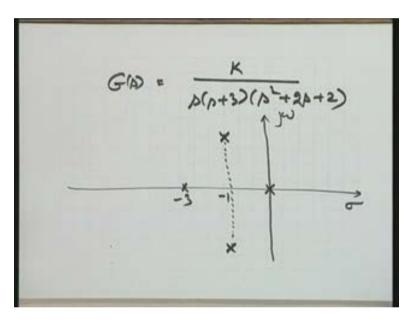
Now you just see in this particular case one two three four there are four poles and therefore there will be four root locus branches K is equal to 0 K is equal to 0 these are the starting points (Refer Slide Time: 17:18) so in this case I know that this particular portion will be on the root locus. I want you to make an attempt first of all to set an idea as to what type of root locus you expect.
