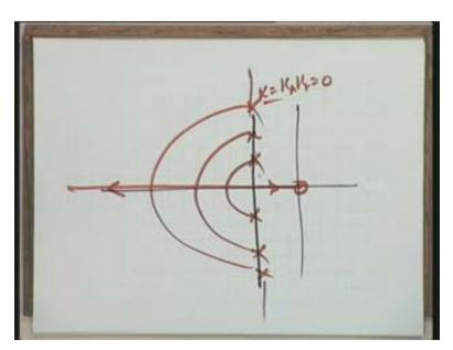
These are the root contours for various values of K A. For every point here K is equal to K A K t is equal to 0, for every point here K is the root locus gain which is equal to K A into K t but each point here or each pair here corresponds to one particular value of K A because this total vertical line is the root locus of the denominator equation as K A is varied so that way
