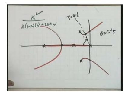
This particular point, well in my notes the calculations have been made for zeta is equal to 0.5 the point is, this particular point is minus point 4 plus minus j 0.7 plus minus j it means these are actually the closed-loop poles of the system. See this particular point: zeta is equal to 0.5 this particular point gives you closed-loop poles of the system and the corresponding
