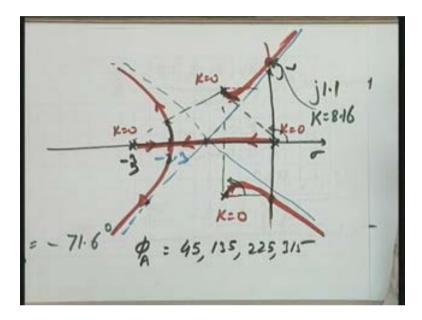
K is equal to 8.16 starting from K is equal to 0, K is equal to 8.16 makes it oscillatory and larger values of k will make the system unstable and the corresponding roots of the auxiliary equation which I have found are plus minus j1.1. So if this point is also available an angle of departure is available in that particular case a rough root locus sketch can be drawn.
