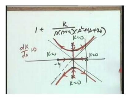
This is the complete root locus plot, you see there are no zeros so all the four branches are terminating at infinity along the asymptotes; all the four branches are terminating and that way you are getting a root locus plot where there are three breakaway points.
