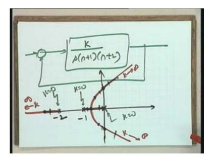
So can we say that this particular diagram has got three branches: for one branch an arrow is shown like this from K is equal to 0 to infinity K is a running parameter, the other branch K is equal to 0 to infinity K is a running parameter, the third branch K is equal to 0 to infinity with this as the third branch as I told you that really scanning this way or this way is immaterial because the two roots are going to be complex conjugate and symmetrical.
