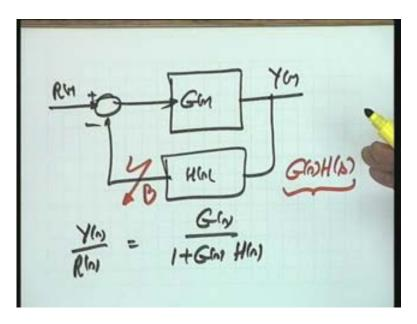
For a unity-feedback system you can very easily see that the open-loop transfer function is same as the forward path transfer function because G(s) is the forward past transfer function that will become open-loop transfer function as well.
