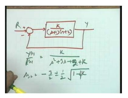
So these are the closed-loop poles of the system: minus 3 by 2 plus minus 1/2 1 minus 4 K under root. Now let us see how does the system behave as the value of K changes from 0 to infinity; after all this is the total change which you can make.
