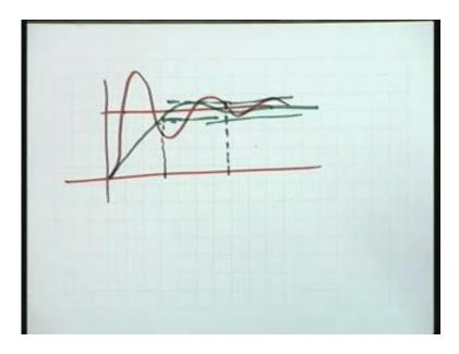
So it depends upon the application you do not want a sluggish initial response in that case you will like to opt for the red curve and if you want the system to settle down quickly, well, the green curve is the optimum choice. So what I want to say is that between the rise time and settling time there may be some sort of decision process involved as is in this particular curve and that depends upon the specific application under consideration.
