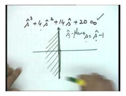
The next point which I have to complete before I let you go because this is a part of the question paper which I have set: G(s) is equal to K this now I take as the feedback system in which there is a parameter K. the parameter K is a design parameter I do not know the value of K and I want to calculate the value of K so that the system remains stable may be a range of the parameters K.
