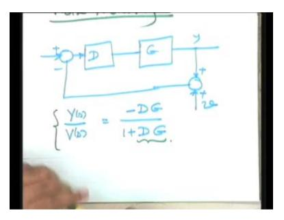
Y(s) over V(s) is equal to what? Yes, I wait for a few seconds just.....minus DG upon 1 plus DG 1 plus DG that is right please. You can just view it as a basic feedback loop; this as a reference input, this as an output this will become forward path transfer function minus D H so it is minus DG over 1 plus DG. Now you see this effect please.
