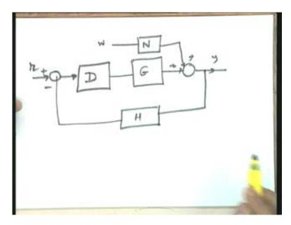
This, we have taken as the error signal e cap and this has been taken as the control signal u. This is the basic block diagram with respect to which the basic characteristics of feedback control systems are being discussed. the transfer function between y and r is given as Y(s) over R(s), we have designated it by M(s) is equal to as you know D(s) G(s) over 1 plus D(s) G(s) H(s). This is your overall transfer function of the closed-loop system.
