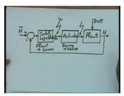
One point I like to mention here; rather one terminology I like to give over here that in this particular case the command signal is a fixed signal, is a constant signal, is not changing with time such a command signal we will refer to this as a set point. This is as per the control system terminology. A set point is a constant command signal. And what is the requirement
