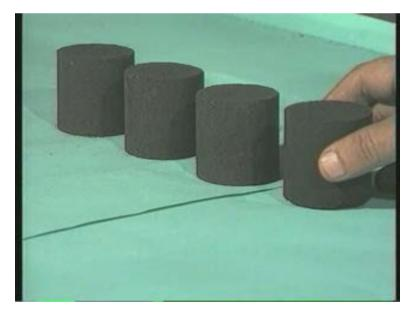
The sand specimen is placed between two fixtures.
