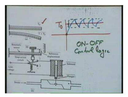
The control logic in this particular case as we will see later is referred to as on off control logic. Because you see in this scheme there is no proportional control, the valve is either on or off, it just takes one two positions and these two positional control is going to give us this oscillating behavior. However, in many feedback control situations this oscillating behavior is acceptable to us.
