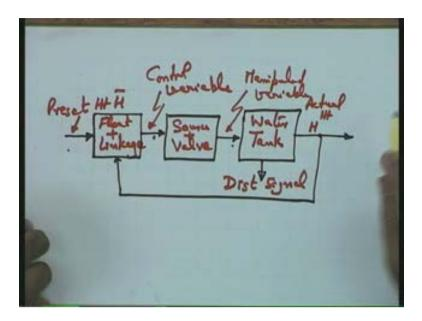
What will happen if this diagram is redrawn into a general format? The format will look like this. So in this particular format I have shown the error detector by this symbolic diagram.
