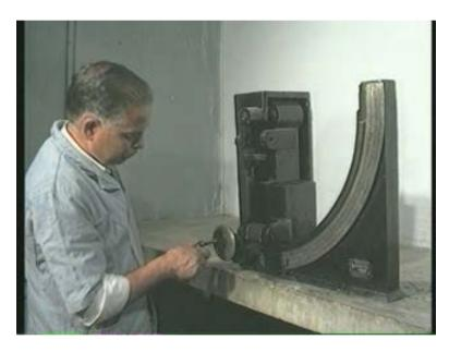
This is the magnetic bit which indicates the strength of the sand at the point of the yielding of the specimen.
