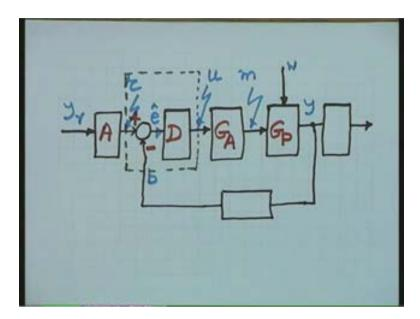
The controlled variable is going to be sensed by the feedback system elements. Note the block feedback system elements, the sensor elements in most of the cases and I use H to represent the feedback system elements. The output of the feedback system elements is the variable b called the feedback signal.
