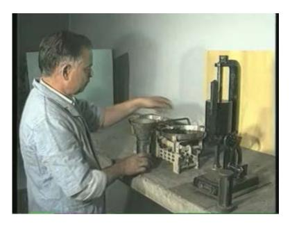
Once the molding sand is prepared it has to be tested for permeability, hardness and strength. So a standard specimen is first made. In this case it is the green sand specimen since it has got water in it. Standard weight is dropped from a fixed height three times.
