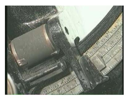
The position of the magnetic bit indicates the green compression strength.
