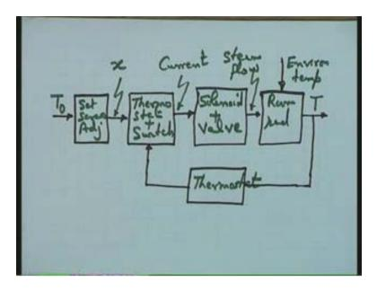
You will please note that in this regulator we have all the ingredients of a feedback structure. The feedback loop the basic feedback loop is here with input as the reference variable and with the output as the controlled variable T. Now looking at the available time I like to conclude my discussion though couple of examples I have yet to give. But before I conclude let me quickly give the basic feedback structure.
