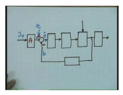
The error signal which is yet to be defined I will like to represent it by the symbol e. Let me proceed further. This error signal is given to this particular block and this particular block corresponds to the control logic block and the control logic let me represent it by D; controller block or control logic block. This total the control logic block and the controller block and the controller block may be referred to as the controller for the system controller for the system.
