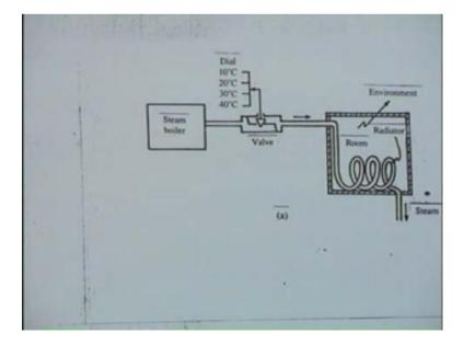
In this particular case you will find that I have a room radiator here. This is the valve which controls the flow of steam into the radiator (Refer Slide Time: 33:15). So, in this scheme as is
