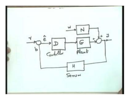
Here is the controlled signal u and here I have taken the reference elements; let me say A as the transfer function of the reference elements and here is y r the command signal or the reference signal which is given to the system. Look at this; this broadly describes the features
