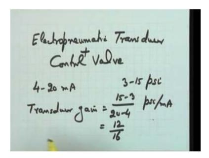
Let me take the two components together and establish a model for this. Please help me. What we will do as far as model of.... we will do the same thing; experimental identification of the transfer function of various components we will do. So, as far as the Electropneumatic
