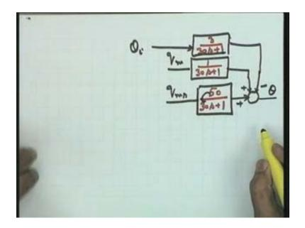
Now this theta here, I can take it on this side, this is the output. Now this output is being sensed and here is my sensor and the sensor transfer function has been taken as 0.16 over 10 s plus 1. This gives me the output here, the sensor output. Here is the control valve, the control valve transfer function we have determined I will recall it 0.1 over 3 s plus 1 where 3 is the time constant of this.
