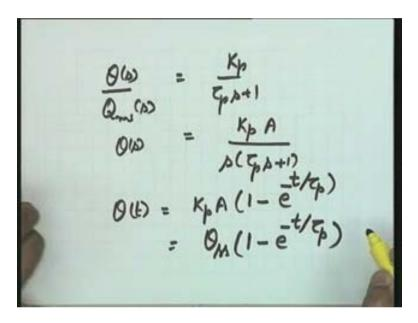
Now let me take the slope at t is equal to 0. This gives me d theta by dt at t equal to 0 is equal to theta ss by tau p at t is equal to 0.
