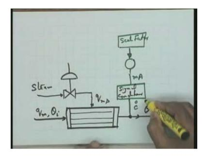
The transfer function or the gain factor of the signal conditioner should be same as the scale factor over here so that the two temperatures can be directly compared in terms of these two signals that is these two current signals so I assume that theta r degree centigrade is my reference and I am assuming milliamperes to be generated as the reference signal. So naturally the error signal is in milliamperes this error signal is now to actuate my controller.
