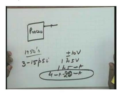
So I will say that the typical signal transmission block diagram will look like this: The process, here is a measured quantity which is a typical process variable, this measured quantity will be fed to a sensor, this sensor will generate an electrical signal now, it could be pneumatic, earlier using suitable force balance equipment pneumatic signals were being
