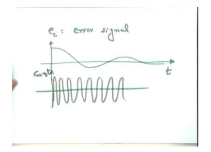
I take this as the carrier frequency for the modulator. So this is my omega c t cos omega c t signal, fine. Let us see what is the nature of the signal, I call that as e m applied to the control phase. This signal will look like, as you know already, a modulated way of this nature the envelop of this particular wave, this, I need your attention at this particular point I will be using this concept in the derivation. This is the envelop of this particular wave which is a low frequency signal e c.
