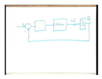
Now please note my point; what I want to say is that I have taken the transfer function between omega and the input to the motor; the input to the motor is control phase voltage. Now that will depend upon this device. I am going to tell you that there may be a device over here which is going to produce a low frequency signal in that particular case that e c is the input and the transfer function which we have derived should be use the wave we have already derived it.
