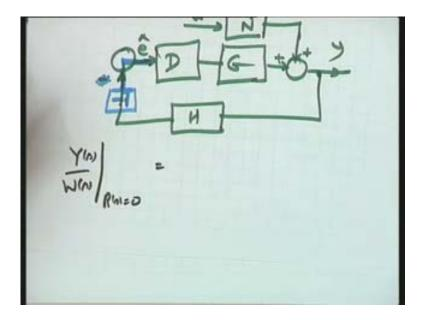
I think there are some errors in all the answers so we can have a quick look at this particular diagram and derive. This minus I take it into this a single minus one and let me complete the loop this way that is the error detector I am removing and putting it as minus 1 here so it means the transfer function now becomes D the block diagram now becomes D G plus plus N w e cap let me put a minus 1 here and this is your H.
