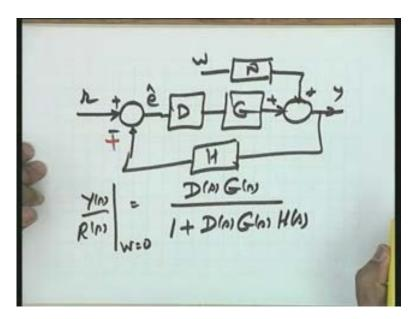
First of all please see, it is a two input one output system. In a two input one output system if you are interested in a transfer function naturally superposition will have to be applied you will have to take one input at a time. So I consider the situation where w is taken equal to 0 and I am
