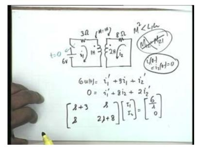
I put t equal to 0 plus, then the left hand side would be 6, would be equal to i 1 prime 0 plus
