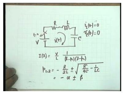
That is, the circuit is initially relaxed and by taking Laplace transform, we had arrived at the solution I of s equal to V by L divided by s minus p 1 times s minus p 2 where p and p 2 are the poles of the circuit and are given by p(1,2) is equal to minus R by 2 L plus minus square root of R squared by 4 L squared minus 1 over L C and we had decided to call this as minus alpha plus
