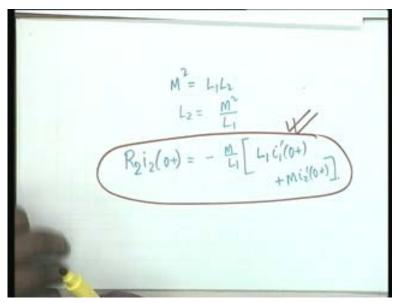
But because M squared is equal to L 1 L 2, I get L 2 equals to, excuse me, M squared by L 1. The fun starts here. Therefore, I can write R 2 i 2 0 plus equal to, I substitute for L 2 and take minus M by L 1 common. Then, what do I get? You see, here I had minus M i 1 prime 0 plus and therefore, if I take M by L 1 common, I shall get L 1 i 1 prime 0 plus and the second one, what do I get plus.
