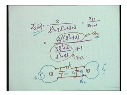
Then, we will see suppose, our function is 2 by s cube plus 3s squared plus 4s plus 2 suppose this is my Z21. The numerator has to be either purely even or purely odd incidentally what kind of a function is this? What kind of filtering does this perform? Where are the 0s?
