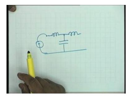
Suppose, we do that what is the problem? The problem is that if you connect a current generator here this pure inductor is in series with a current generator and is absolutely ineffective.
