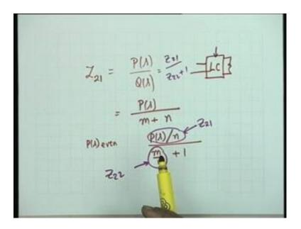
Now, the synthesis procedure should be quite simple I will illustrate this with Z21 that it is given as P of s by Q of s, where P of s is either purely even or purely odd. Because, we want to realize this is an LC network terminated in 1 Ohm resistance. So, P of s is purely even or purely odd and Q of s must be Hurwitz. So, what we do is we write the, we separate the even or odd parts.
