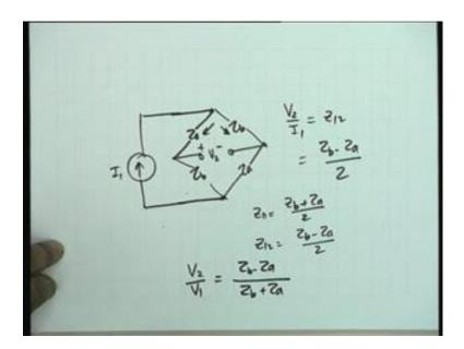
What we have is Za Zb this is Za and this is Zb we apply a current a generator I1 here and we measure the voltage V2 here plus minus. And V2 by I1, shall be equal to Z12 you see V2 by V2 is this voltage minus this voltage which simply means, that it is Zb minus Za divided by 2 why because, the current divides into 2 equal parts I1 by 2 and I1 by 2 we did this earlier.
