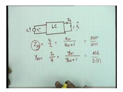
That is an LC network, LC network terminated in a resistance this is the most useful form of network synthesis, in practice most useful form. The it can be either a voltage generator or a current generator and the response could be either the voltage. We assume the termination to be 1 Ohm we normal the termination to 1 Ohm and this current is I2. So, we can have a transfer function like let us, say V2 by I1 what would you call this transfer impendence.
