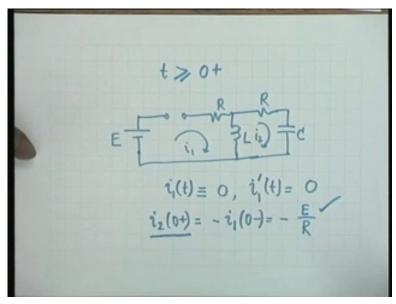
Now regarding the primes, regarding the primes, what we have to do is, you have to find out the circuit at t greater than equal to 0 plus. Let us look at this circuit, t greater than equal to 0 plus. There is this voltage source E and then the switch has been thrown open, then a resistance R and inductance L. This is i 1, and then another resistance R and the capacitance C and this is i 2,
