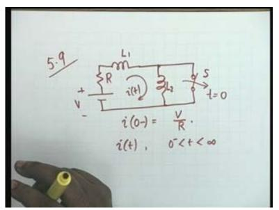
5 point 9 is also a peculiar problem. 5 point 9 says that you have a resistance R, a battery V plus minus, an inductor L 1 and then an inductor L 2. Across L 2 there is a switch and the switch was initially closed and thrown opened at t equal to 0. For the circuit shown the switch s is opened t equal to 0 after this circuit had been in steady state, which means that, if this current is i of t then i of 0 minus would be simply equal to V by R.
