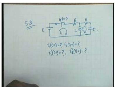
The problem is a network is given like this E, switch s is thrown out at t equal to 0, that is, it was closed earlier, it have been opened now and then you have a resistance and inductance Lm another resistance R and a capacitance C. This is the network. This current is i 2 and this current
